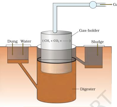
Figure 8.8 A typical biogas plant
